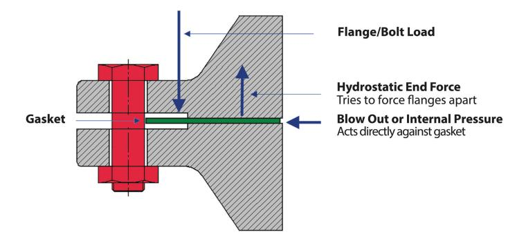
The flange pressure, or minimum seating stress, necessary to accomplish this is known as the "Y" factor. This flange pressure must be applied uniformly across the entire seating area to achieve perfect sealing. However, in actual service, the distribution around the gasket is not uniform. The greatest force is exerted on the area directly surrounding the bolts. The lowest force occurs mid-way between two bolts. This factor must be taken into account by the flange designer.
