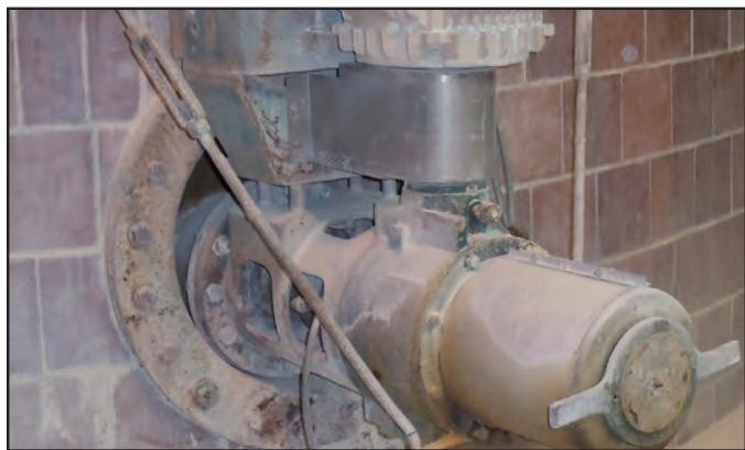
One of four slurry tank agitators installed with Inpro/Seal AM Solutions shaft seals to eliminate product loss and decrease maintenance costs.
